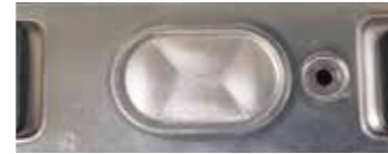
Explosion-proof valve welding
